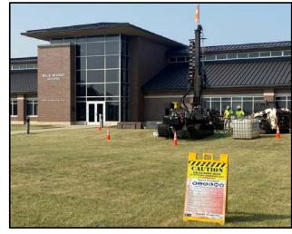
A drilling rig is used to collect soil and groundwater samples in 2021. The building shown was built over the former fire station where fire-fighting foam was used, stored, and spilled.
